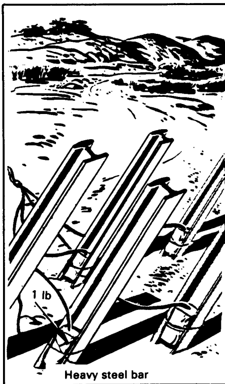
FIGURE 5-14. CHARGES PLACED ON BEACH OBSTACLES
